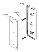
Replace cover by pressing snap latches into place.
